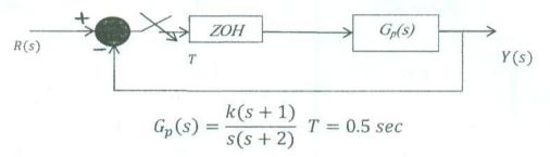
Using Jury's test, determine the range of *K* for the system to be asymptotically stable.
