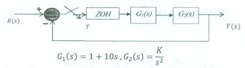
Find the range of *K* for the system to be stable using root locus.
